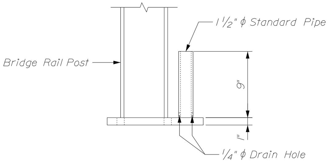
~ MODIFIED BASE PLATE ELEVATION ~
